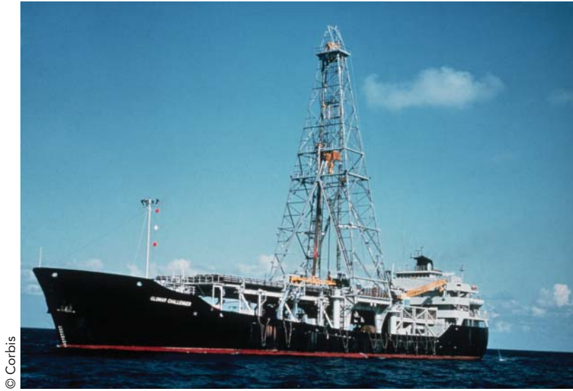
FIGURE 1-7 The Deep Sea Drilling Vessel Glomar Challenger . The prominent derrick at midship allows roughnecks on the drilling floor to hoist lengths of pipe upward, and then add that new length of pipe to the pipe already “in the hole.” In 1970, while operating in the Mediterranean, the Glomar Challenger brought up drill cores indicating the Mediterranean was once a desert.
